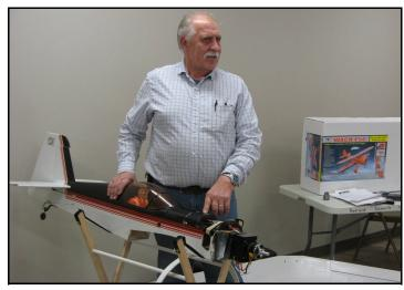
**Jeff Slater** brought a Goldberg Sukhoi 26 that he bought at an estate sale. He is installing an E-Flite 110 motor and two 4s-4000 batteries for power.
