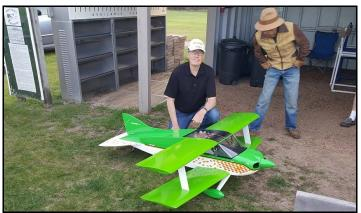
**Bob Proulx** brought a scratch built Hyper Bipe AKA Sorell SNS 7. Bob enlarged plans of a smaller version to true 1/4 scale. The unusual shaped airplane has a 65-inch wing span with the
