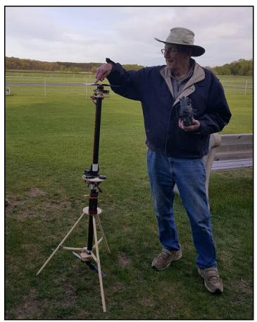
**Dave Willemssen** brought his v2.0 of his "Push me, Pull you" on a stick. The unusual flier uses articulated 650kv motors with 15 X 5.5 props, which are at the top and bottom. For flight stability, it uses "Drone" attitude controllers capable of altitude hold mission flights. Collapsible tripod style legs allow the 5.5 lb craft to stand upright. Additional testing and tuning will need to be done in a wind free area.
