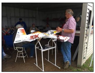
Jeff Slater brought a CAP 232 foamy by Flex Innovations. Jeff feels the \$440 price tag and less than an hour to assemble make it a worthwhile investment. Much of the set up is performed at the factory including the Aurora 8 receiver and Potenza 6030 500 KV motor. Weighing in at 5 pounds, it also has selectable gyro steps to go from mild to wild. 5-minute flights are the norm and it is illuminated for night flying.
