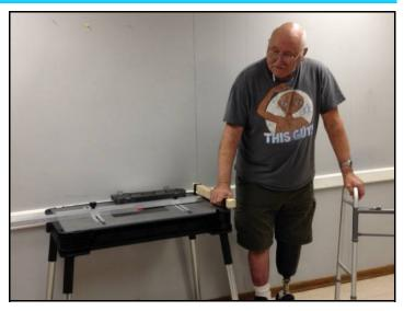
Stan Zdon brought a Husky Tools portable workbench that he modified to hold his airplanes for maintenance and starting. Adjustable wheel chocks position different length aircraft to a secure starting position.
