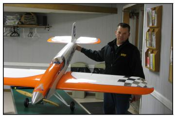
Jason Korst brought a Balsa USA 88 inch Smoothie. His first Balsa USA kit, the excellent laser cut parts made him smile. Powered by a 30cc DOE engine, controlled by HiTec radio system. The airplane has functioning flaps. Weight in the 12 to 14 pound range.
