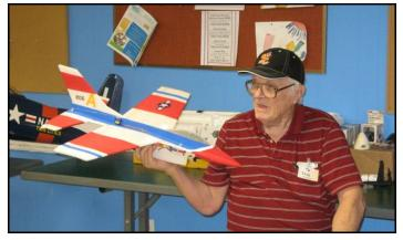
**Don McGillivray** bought in a homemade foam plane that he scaled down to 2/3 size of the plane he bought. He put a 55mm outrunner ducted fan motor using a pair of 430 MA LiPos for power. It has flown twice and he says it's a great flyer. Weight is 11 oz with 8 oz of thrust.
