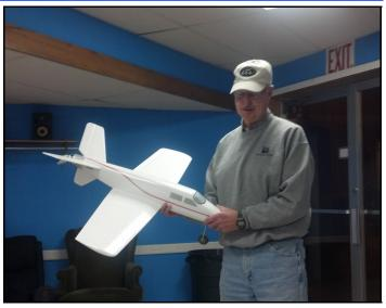
Ron Fichtner showed us his scratch-built from RCM plans. It is called the "FireFox", it weighs 3 pounds and it is powered by a 15 size electric motor.
