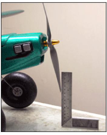
Propellers can be out of alignment by manufacture, or from over tightening - especially with wood propellers. The problem is exacerbated in large propellers with multiple holes. Each bolt should be tightened the same amount to prevent a tracking problem.
